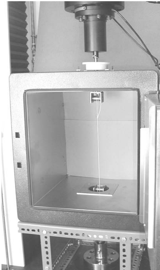
Fig. 2 Test set-up showing oven installed in test machine
